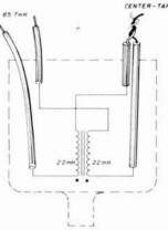
fig. 1. The schematic diagram shows the inductor connections inside the potted case, and the external connection (series-aiding) required for 85.7 mH. The photograph shows the unsatisfactory results of removing the inductor from its potted container. The leads are connected in series aiding for 85.7 mH.
